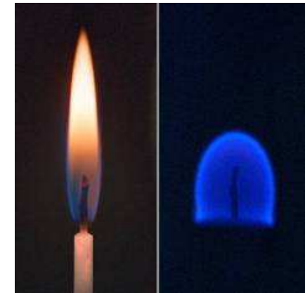
A candle flame in Earth's gravity (left) and microgravity (right) showing the difference in the processes of combustion in microgravity.
